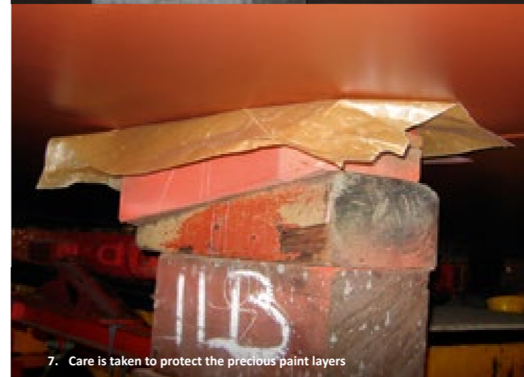
6. Pillars, sandboxes, blocks and wedges support the ship under construction
